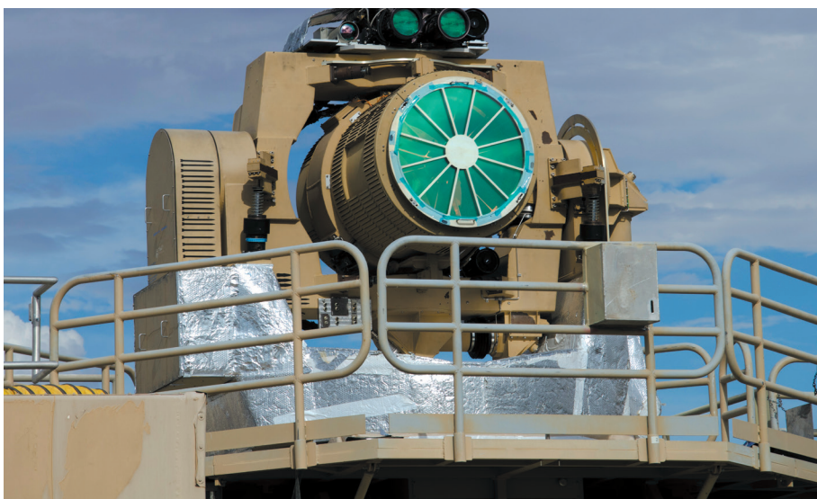
The Joint High Power Solid State Laser system's beam director. The JHPSSL was originally built with the goal of advancing U.S. laser technology and not intended for deployment. Today, the system is used to conduct test missions looking at laser system capabilities.
