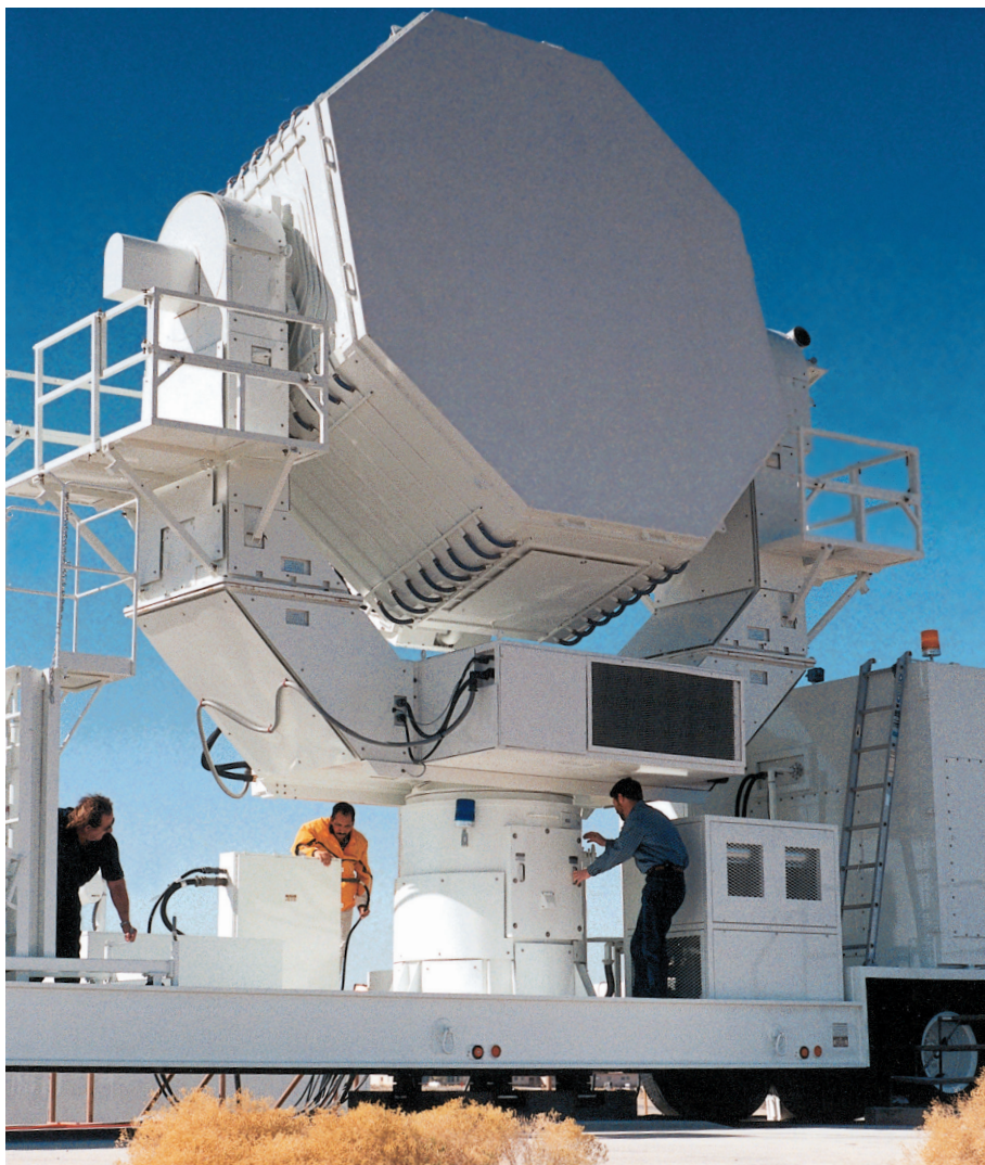
Radar specialists work with the Multiple Object Tracking Radar, which can track as many as 40 objects at a time.
