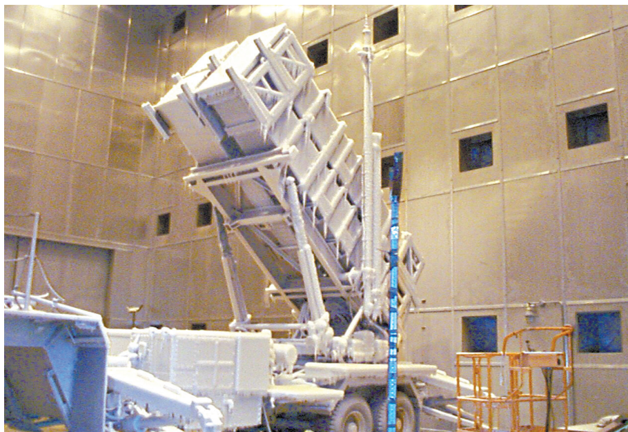
A Patriot Advanced Capability 3 launcher undergoes cold testing in a White Sands Missile Range climatic chamber.
