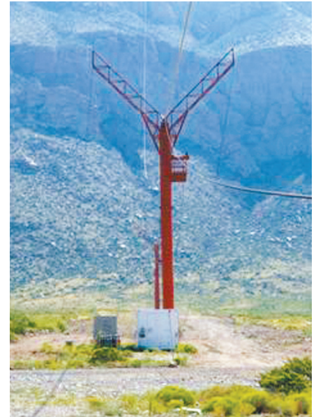
The Aerial Cable Range is a 3-mile-long Kevlar cable strung between two mountain peaks from which targets can be suspended for test purposes.
